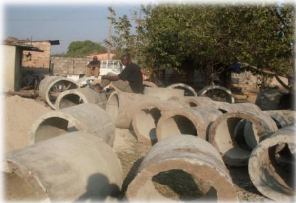
CAIP PROJECT: 900mm and 600mm Ring culverts ready for to the Mansa Municipal Council for CAIP Projects. July, 2011
