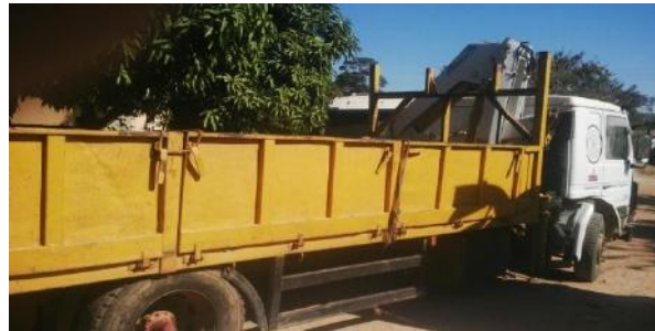
21 Ton Truck Mounted with a 7.5 Ton Crane
