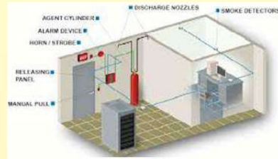
Fire Suppression System
